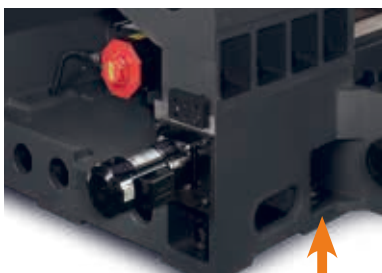
Additional pads for column supporting
